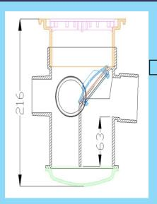
Fool proof sealing arrangement for gases as compared to other floor traps in the market.
