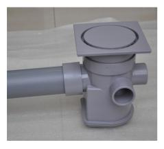
Full bore optional dual outlet, for 63 mm or 75 mm outlet. Outlet not blocked to create water seal, unlike other models available in the market.
